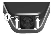
Press the two locks 1 for the housing cover on the underside of the Wallbox upwards.
