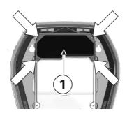
1. Undo the four screws used to secure the terminal panel cover **1**.
