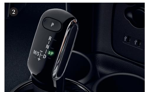
① MINI Driving Modes. ② Electronic gear selector lever for 7-gear double-clutch transmission.
